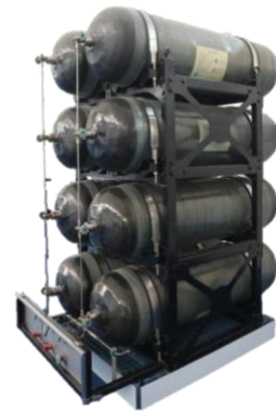
Fig 2 Current COPV design to store 700-bar hydrogen.
