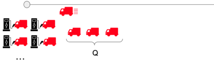
Fig. A3: Truck arrives at truck stop with all chargers in use, and a queue of length Q trucks waiting to charge.
